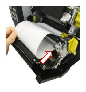
6. Feed the leading edge of liner through the peel-off module slot as indicated.
