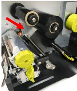
2. Slide the ribbon off to release the ribbon on the ribbon rewind spindle.
