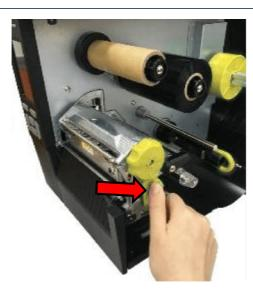
3. Push the Print head release lever to open print head mechanism.
