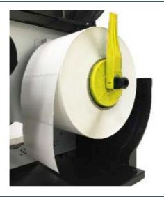
3. Place the media roll on the label supply spindle and use label roll guard to fix it.
