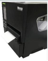
5. Close the print head mechanism and press the FEED button to test.
