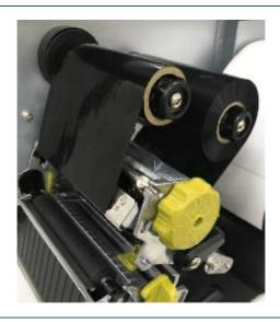
5. Stick the ribbon leader onto the paper core. Keep the ribbon flat and without wrinkle.
